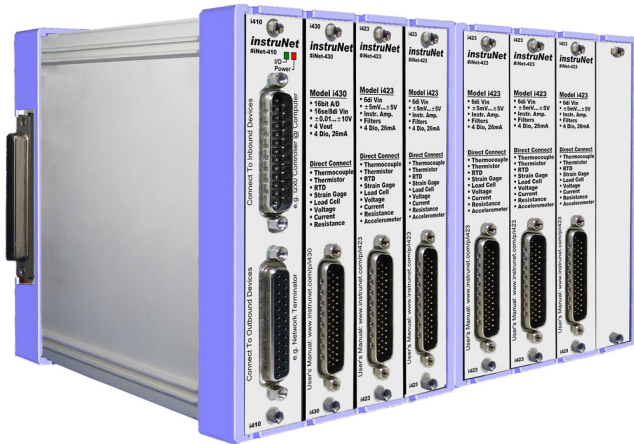
i60x can digitize concurrently with instruNet i555 card cage system; which supports 4, 8, 12 or 16 slots of analog/digital i/o hardware.
